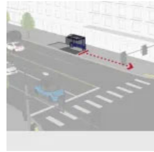
Computer generated graphic of a bus with an in-lane bus stop
